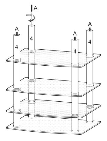
Screw long rods (A) into cylinders (4).
